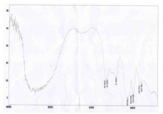
Figure 2. IR of extracted phytic acid
